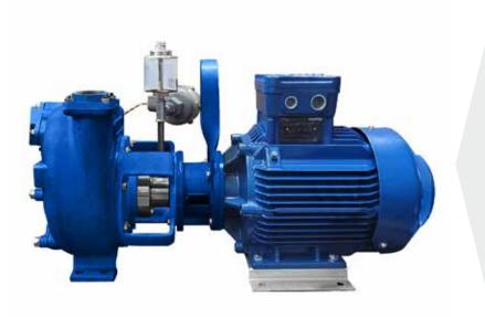
Suction port Threaded - 2" ISO 228 (BSP) Delivery port Threaded - 2" ISO 228 (BSP) Qmax 46 m<sup>3</sup>/h - 767 l/min (202 USgpm) Hmax 60 m (197 ft) Solids handling 14 mm (0.55") Motor power 11 kW - 15 HP Motor type **IEC** standard **Cast iron frame** Motor brand CEMP Weight 279 kg (615 lb)
